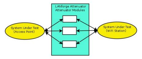
The LANforge attenuator sits between two RF systems, often a WiFi AP on one side and WiFi Station on the other. The attenuator and WiFi stations are connected by shielded SMA-Male cables. Adjust the attenuation as desired either with the LANforge GUI or direct access over serial.
