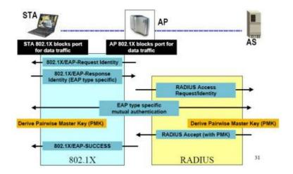
Once the PMK is generated the 4-way handshake occurs then the PTK is generated which is used for encrypting the further data.
