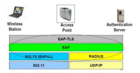
Initially, during the connection first the station sends a probe request to the Access point then the AP sends the probe response having the RSN IE stating the capabilities of the access point like the security it supports etc. Then the client gets authenticated and associated to the AP.
