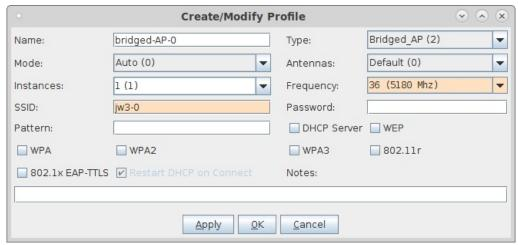
D. Once you have saved and selected the Scenario, click **Apply Scenario** and then click **Build Scenario**. The APs will be created, bridge devices will be created and will contain the APs and the Ethernet ports selected in the scenario. The Access Point devices will be started as part of the build process, so the system is now ready to be used. You can also make further modifications to the AP configuration by modifying the vap interfaces in the Port-Mgr tab of the LANforge GUI.
