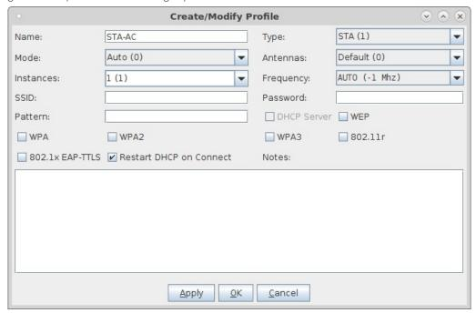
G. Configure a Chamber View Scenario and add the STA profile (mapped to desired wiphyX radio and DUT). Add an upstream profile mapped to DUT LAN side (or possibly WAN side if that is more appropriate for your DUT). Choose the appropriate quantity of stations for your test case.
