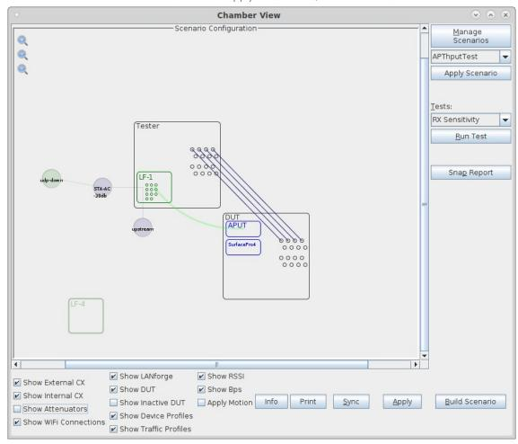
B. Select the **WiFi Capacity** test and click **Run Test**. You should see the WiFi Capcity Test configuration window pop up. The Ports are normally selected properly based on the Scenario, but you may need to adjust them depending on your goals and scenario. Select the desired throughput and any other configuration changes from the defaults:
