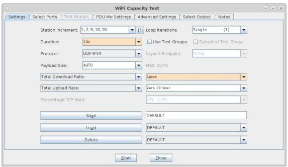
C. When the configuration is complete, click the **Start** button (which will change to 'Stop' once start is clicked) to start the test. An interactive report window will be created and will be updated as the test runs. In this particular test, the results are a it unexpected. Normally rate starts off high and slowly decreases after 5 or 10 stations are active. In this case, we see a falloff after 10, but then it recovers at 60.
