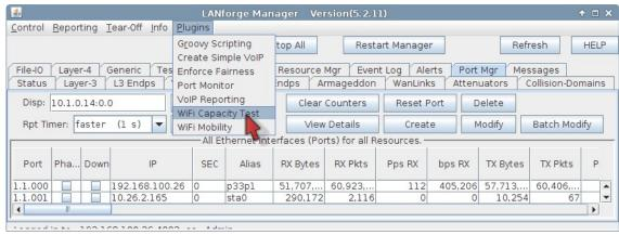
A. Highlight free ports that you want to add to the test, this includes the upstream port eth1 and the virtual stations sta0 - sta127.
