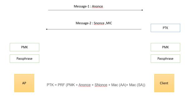
With Snonce, from Message 2 AP will also generate PTK and calculate the MIC internally and compare with the MIC being sent in the Message 2.
