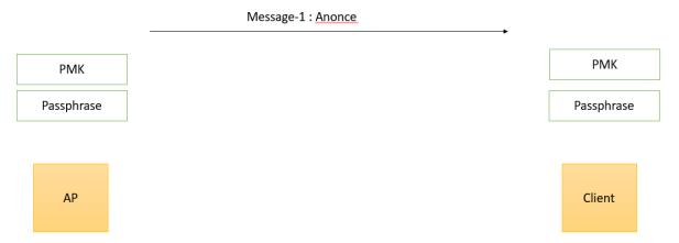
After the 'message 1' has been sent from AP to the client. The client will calculate the PTK using a pseudo random function.
