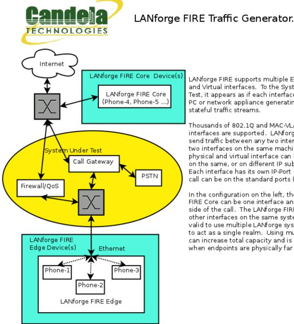
LANforge FIRE supports multiple Ethernet and Virtual interfaces. To the System Under Test, it appears as if each interface is a separate PC or network appliance generating independent stateful traffic streams.
