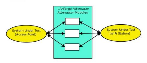
The LANforge attenuator sits between two RF systems (often WiFi AP on one side and WiFi Station on the other. Connect shielded RP-SMA Plug cables between the Attenuator and WiFi Stations. Adjust the attenuations as desired using Attenuator knobs and/or use a program to adjust the values over the USB-Serial connection.
