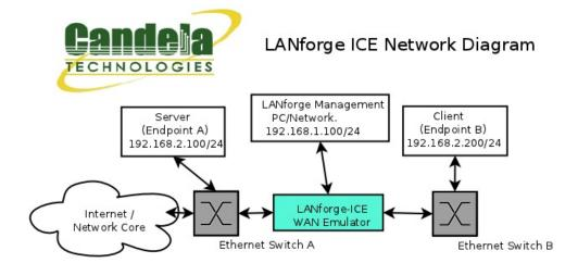
This diagram shows how one might use LANforge ICE to emulate a Wide Area Network between a Server and Client. When the Client communicates with the Server, the traffic will flow through the Ethernet switches and then through LANforge ICE. LANforge ICE will enforce the rate limitation and other network emulation as configured. The Client and Server are on the same subnet. For a simpler configuration, the Client and Server can be directly connected to the LANforge ICE system.
