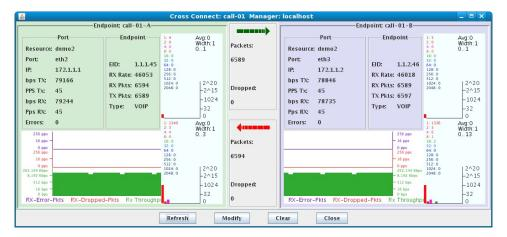
The busy graphs on the right of each panel display latency and jitter distributions for each endpoint over the last 30 seconds. LANforge detects latency with the RTCP protocol. Jitter is determined from the timestamp on the received RTP packets. Note that the jitter calculation is made before the packet is processed by the RTP Jitter buffer.
