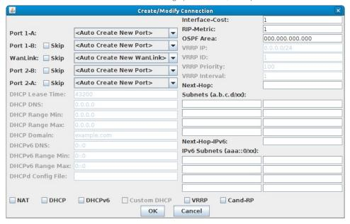
You can choose up to 4 ports and one WanLink to be part of this connection. The number and combination of ports/WanLink selected changes the behavior significantly. In the example below, it is assumed that Port-1 will be the 'outside' port, but Router Connections do not have an inherent direction...it all depends on how you configure it.
