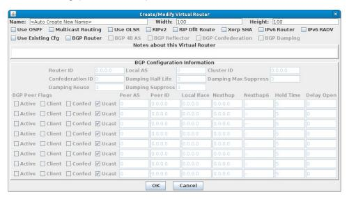
LANforge will generate a name automatically unless one is entered. The name, graphical size, notes field and other router configuration flags can all be modified when created or at a later time. The virtual router will use simple subnet routing rules unless otherwise directed. Xorp must be installed before using the following routing features: OSPF, Multicast, RIP, Xorp SHA, or BGP.
