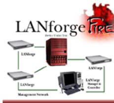
LANforge FIRE generates network traffic at various speeds with the ability to monitor packets for throughput and correctness. LANforge FIRE sits on the edge of your network and tests your network core.
