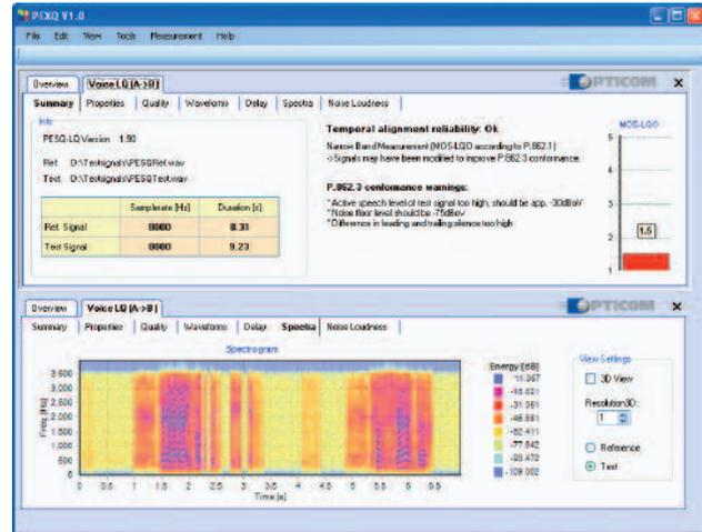
PESQ Analysis of Listening Quality (upper diagram) with Spectrogram of test signal (lower diagram). Note the easy configurable tab selection for multifaceted result views.
