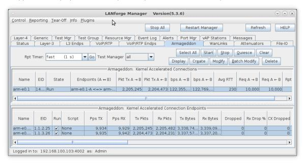
A. **NOTE**: Delay for Armageddon connections is measured in microseconds (us) and in this example, the system experiences about 39us of delay when sending to itself.
