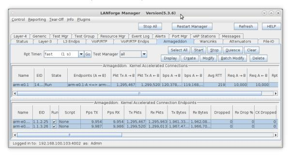
C. In this example, this system (1.8GHz Intel Atom D525, 6 onboard 10/100/1000 ports) is capable of reaching 81,000pps with 1514byte packets or, an equivalent speed of about 990-1005Mbps bi-directional.
