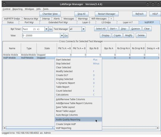
B. Select the required configuration and **Start** the monitoring.
