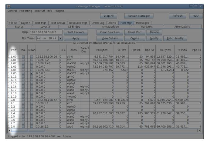
For now, assume the shelf number will always be 1. The Resource number will refer to the LANforge machine ID as reported on the Status tab. The Port ID is only unique within a LANforge machine. The Port ID also refers to hardware in a machine: radios get a third decimal. The fourth decimal refers to either endpoints or connections.
