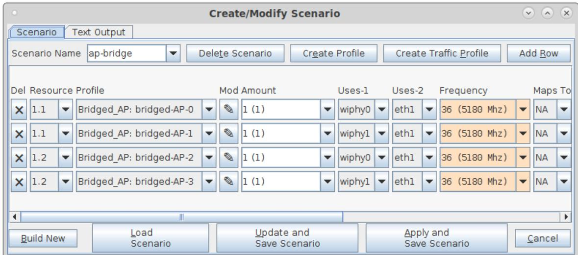
C. This example uses 4 different bridged-AP profiles. Each profile is the same except that it has a different SSID.
