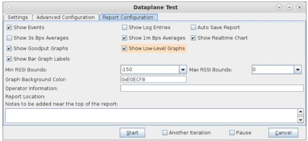
D. When the configuration is complete, click the **Start** button (which will change to 'Stop' once start is clicked) to start the test. An interactive report window will be created and will be updated as the test runs.
