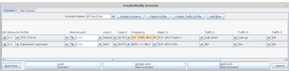
A. Open Chamber View by clicking on the 'Chamber View' button in the LANforge-GUI. Load appropriate scenario. Apply the Scenario, then Build the scenario.
