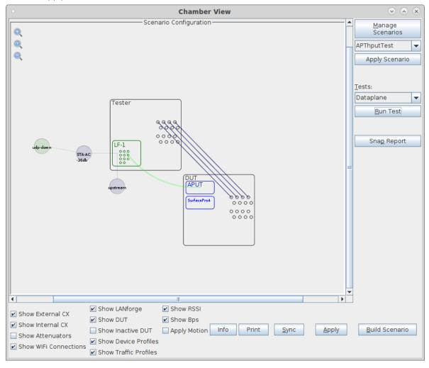
B. Select the **Dataplane** test and click **Run Test**. You should see the Dataplane Test configuration window pop up. It will remember the last configuration for most fields. Select the DUT and WiFi station device, and select the combinations of traffic types and packet sizes you wish to send.:
