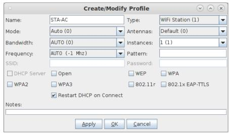
G. Configure a Chamber View Scenario and add the STA profile (mapped to desired wiphyX radio and DUT). Add an upstream profile mapped to DUT LAN side (or possibly WAN side if that is more appropriate for your DUT).
