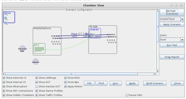
B. Select the **Hunt** test and click **Run Test**. You should see the Hunt Test configuration window pop up. It will remember the last configuration for most fields. Select the DUT and WiFi station device, and select the combinations of traffic types and packet sizes you wish to send.
