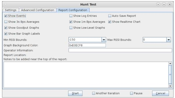
E. When the configuration is complete, click the **Start** button (which will change to 'Stop' once start is clicked) to start the test. An interactive report window will be created and will be updated as the test runs.
