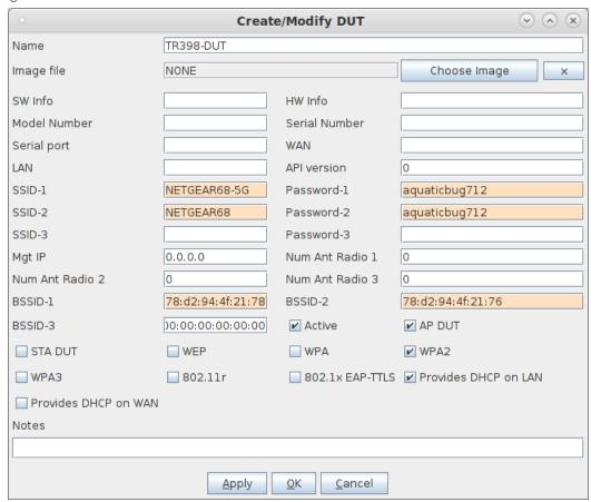
C. Create a chamber object to hold the DUT, and add the DUT to that chamber. If you have no chambers, you can create a fake chamber, but your test will not be isolated and may not function as desired.
