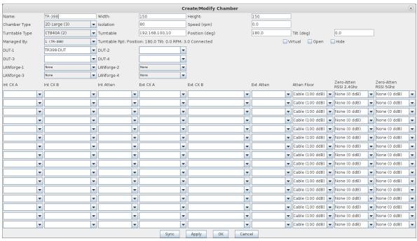
D. Create a chamber object to hold the LANforge system, and add the LANforge to it. Add connections from this chamber to the DUT chamber, specifying the proper Attenuator modules. Please view our other cookbook on setting up attenuator connections in LANforge.
