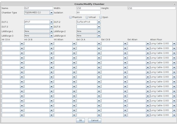
D. Create a chamber object to hold the LANforge system, and add the LANforge to it. Add connections from this chamber to the DUT chamber, specifying the proper Attenuator modules. Please view our other cookbook on setting up attenuator connections in LANforge.
