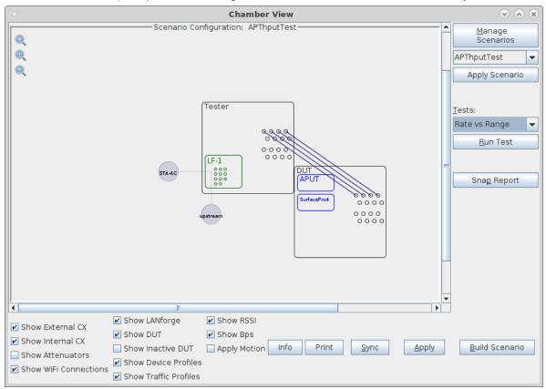
B. Create a Device Under Test (DUT) Profile that matches your AP. The BSSID is important to configured so that LANforge knows when it is connected to the correct AP.
