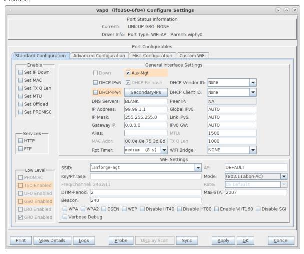
C. On the other resources, configure the wlanX interface to connect to the AP on the manager system, and select the **Aux-Mgt** checkbox.
