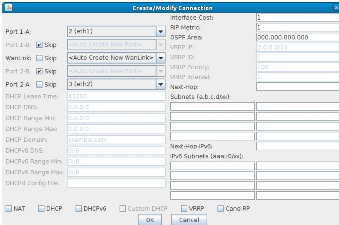
A. Select the Skip checkboxes on **Port 1-B** and **Port 2-B**.
