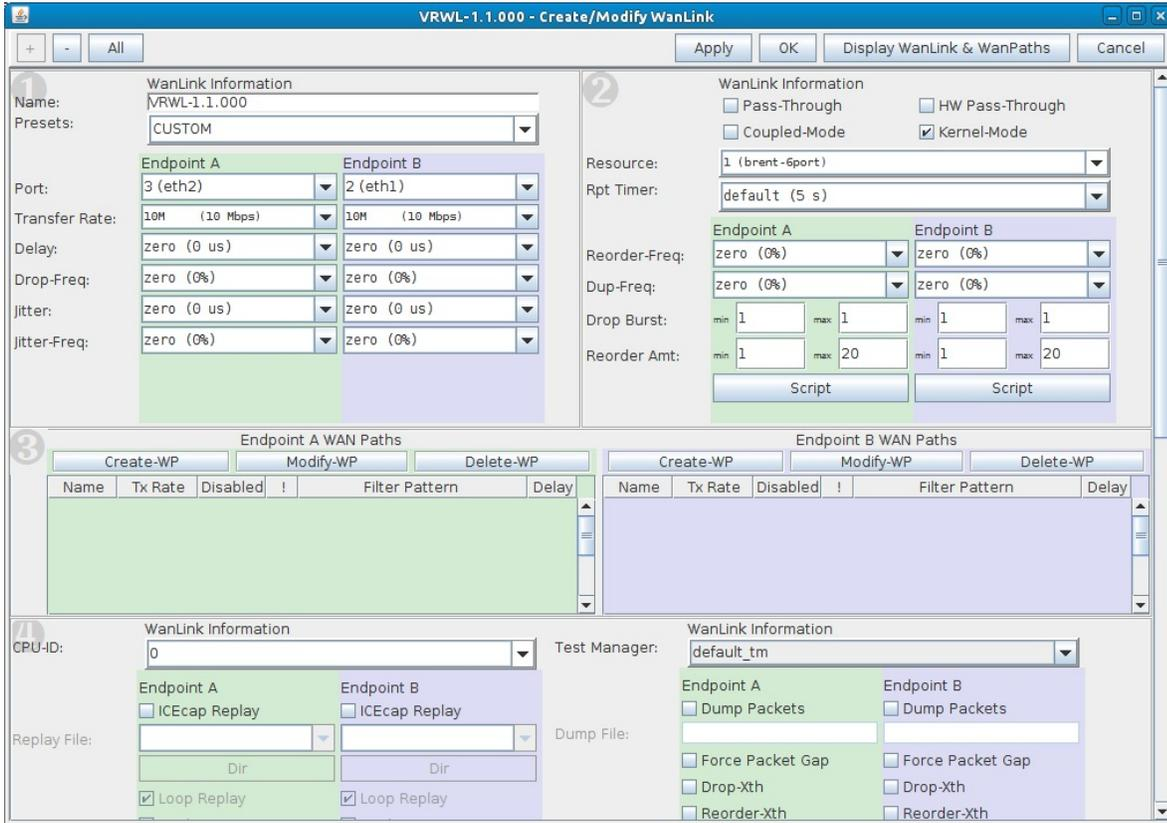
A. Set the Transfer Rate to **10Mbps** for **both** endpoints.
