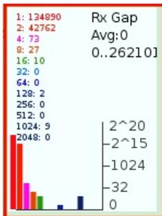
A. The colored numbers on the left side of the colon represent time in milliseconds. The right colored numbers represent the number of times a sequence gap reached the particular time on the left side.
