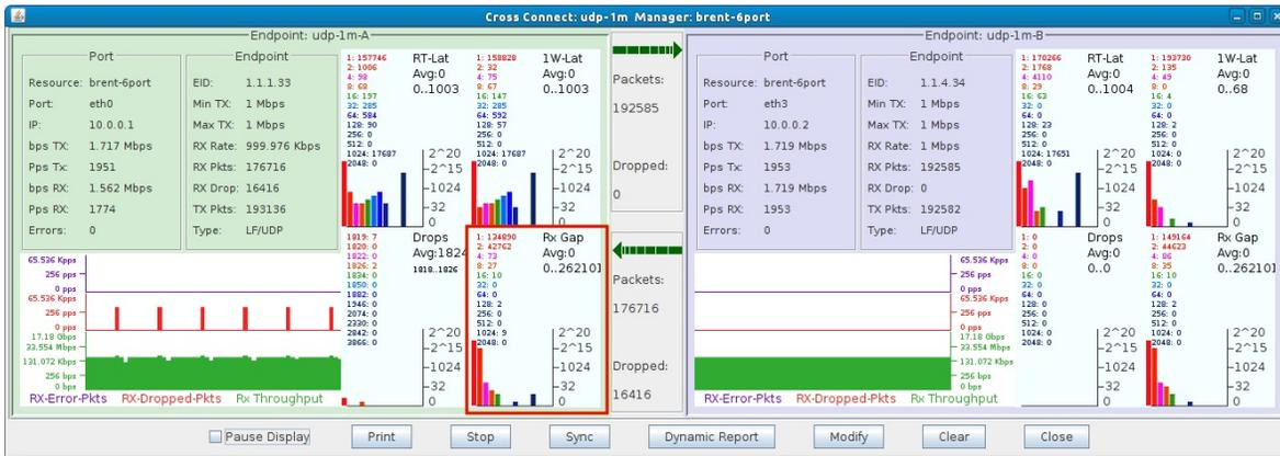
B. The **Rx Gap** graph is highlighted in the below screenshot. The Rx Gap for Endpoint B doesn't show one second sequence gaps because that side of the WanLink was not scripted.
