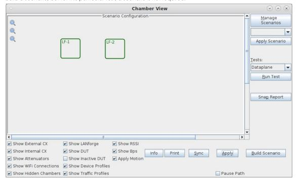
B. Select the **Dataplane** test and click **Run Test**. You should see the Dataplane Test configuration window pop up. It will remember the last configuration for most fields. Select the two 10G ports and the combinations of traffic types and packet sizes you wish to send:
