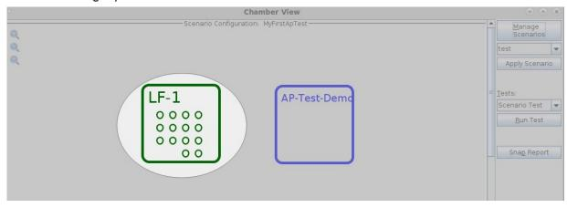
6. All active LANforge systems will automatically appear in Chamber View. Select the unit being used in the test and drag to the middle of the canvas next to the AP under test. The small circles inside the LANforge box represent the SMA connectors. The columns of circles represent the individual radios in the system For instance, in the screenshot about LF-1 has 4 columns of circle indicating 4 radios. The first two are 3x3 radios and the second two are 4x4 radios with 4 circles each.
