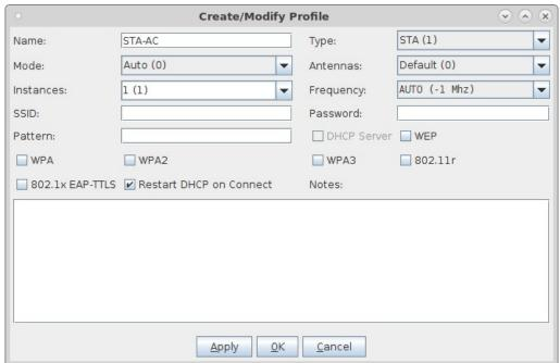
G. Configure a Chamber View Scenario and add the STA profile (mapped to desired wiphyX radio and DUT). Add an upstream profile mapped to DUT LAN side (or possibly WAN side if that is more appropriate for your DUT).
