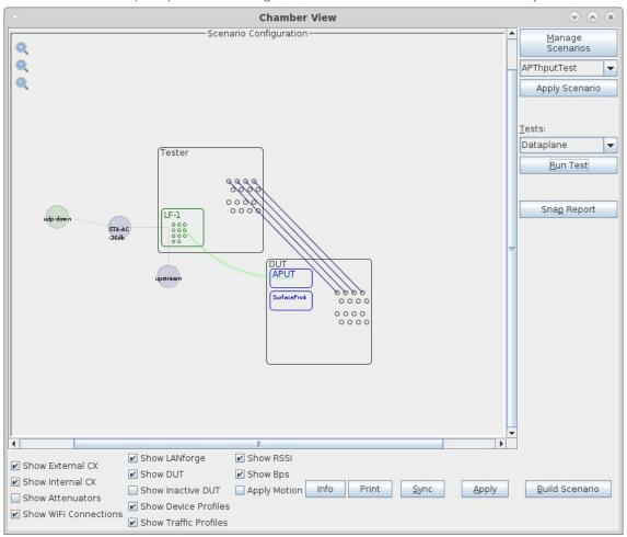
B. Create a Device Under Test (DUT) Profile that matches your AP. The BSSID is important to configured so that LANforge knows when it is connected to the correct AP.
