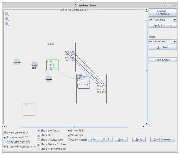
B. Select the **RX Sensitivity** test and click **Run Test**. You should see the RX Sensitivity Test configuration window pop up. It will remember the last configuration for most fields. Select the DUT and WiFi station device, and select the combinations of traffic types you wish to send.:
