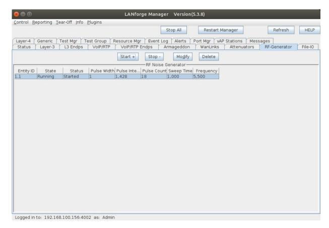
5. When the CT712 is activated, the Status will show Started and the HackRF-One device's TX LED should show a red light. The AP under test should detect RADAR within 10 seconds, change to an available channel and not be able to use the previous channel again for 30 minutes.
