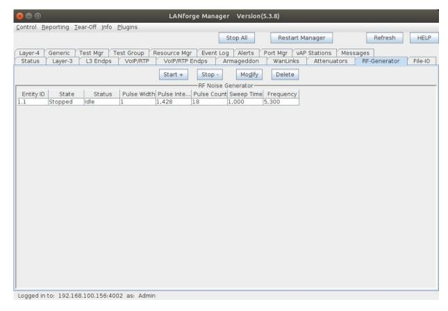
3. Select a FCC RADAR type preset button or enter specific values to set the desired pulse characteristics, then set the transmit frequency, then select OK.
