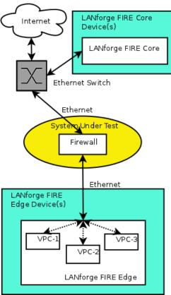
LANforge FIRE supports MAC-VLAN virtual interfaces. To the System Under Test, it appears as if there are multiple PCs sitting inside the LANforge system generating independent traffic streams.
