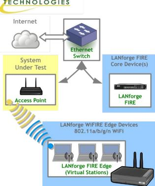
LANforge WiFIRE supports 802.11 Virtual Stations and Access Points\*. To the System Under Test, it appears as if there are multiple PCs sitting inside the LANforge system generating independent traffic streams over Wireless NICs.
