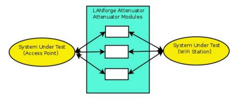
The LANforge attenuator sits between two RF systems, often a WiFi AP on one side and WiFi Station on the other. The attenuator and WiFi stations are connected by shielded SMA-Male cables. Adjust the attenuation as desired either with the LANforge GUI or direct access over serial.
