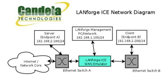
This diagram shows how one might use LANforge ICE to emulate a Wide Area Network between a Server and Client. When the Client communicates with the Server, the traffic will flow through the Ethernet switches and then through LANforge ICE. LANforge ICE will enforce the rate limitation and other network emulation as configured. The Client and Server are on the same subnet. For a simpler configuration, the Client and Server can be directly connected to the LANforge ICE system.
