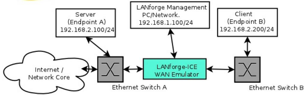
This diagram shows how one might use LANforge ICE to emulate a Wide Area Network between a Server and Client. When the Client communicates with the Server, the traffic will flow through the Ethernet switches and then through LANforge ICE. LANforge ICE will enforce the rate limitation and other network emulation as configured. The Client and Server are on the same subnet. For a simpler configuration, the Client and Server can be directly connected to the LANforge ICE system.
