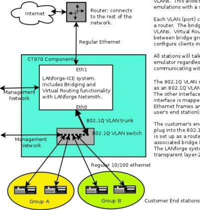
The LANforge-ICE system can have a large number of 802.1Q VLAN interfaces. Each physical port on the VLAN switch maps to a separate VLAN, and the LANforge-ICE WAN emulation is applied to specific VLANs. This allows a large number of distinct WAN emulations with a single LANforge machine.
