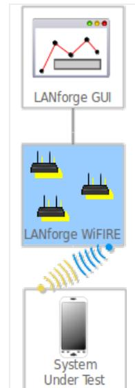
1. Setup a single virtual access point on each wifi NIC for at least two NICs and configure them for the same channel and SSID.
