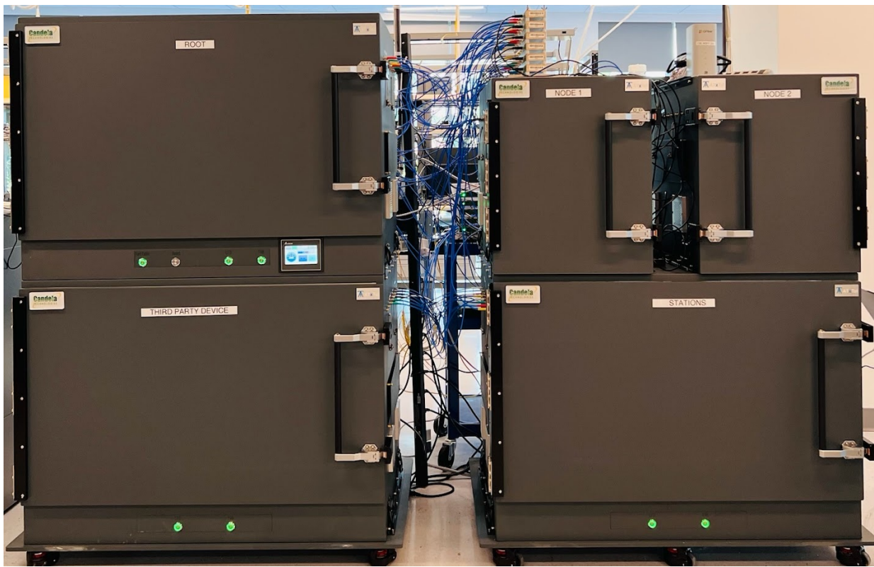
TR398 issue-4 with 2 mesh extenders in single 80db chamber stack with side-mount attenuators and custom cable lengths for clean cabling. 32 Intel be200 Radios plus 1 tri-band tri-concurrent virtual station radio.
