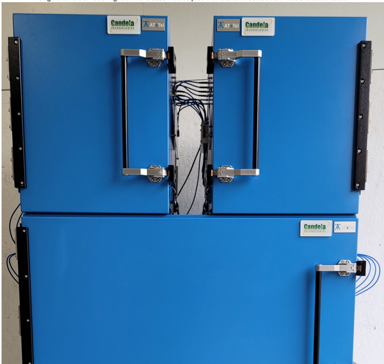
TR398 issue-4 with 2 mesh extenders in single 80db chamber stack with side-mount attenuators and custom cable lengths for clean cabling. 32 Intel be200 Radios plus 1 tri-band tri-concurrent virtual station radio.
