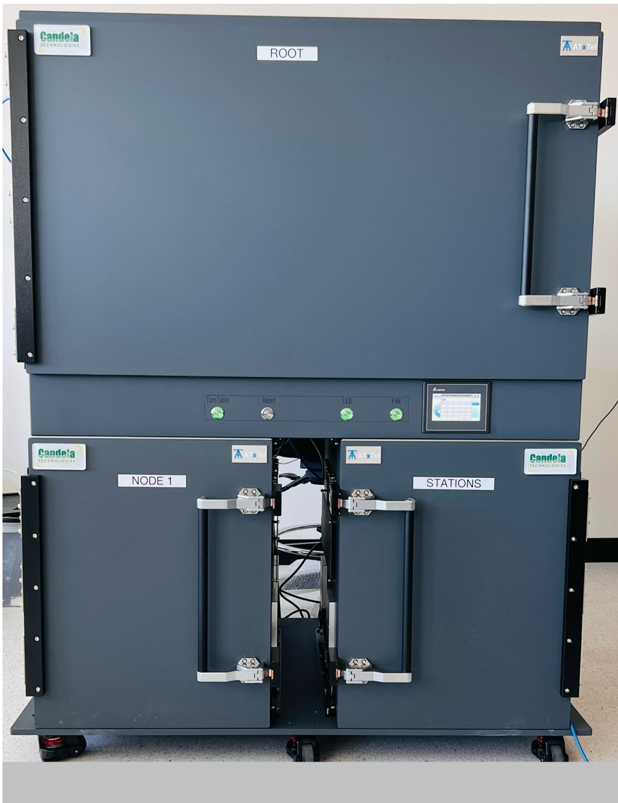
TR398 issue-4 with 2 mesh extenders plus 3rd-party devices chamber, 32 Intel be200 Radios plus 6 virtual station radios.
