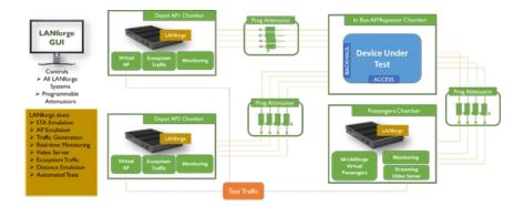
All chambers are connected using programmable attenuators. The setup allows 100s of emulated passengers connecting to the AP under test while roaming the AP under test in the bus between the 2 Depot APs. LANforge can generate emulated HD video streaming and other traffic flows and report details of the end-user experience.
