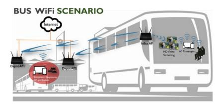
If we take buses as an example, the AP in the bus needs to provide good quality of experience to all the passengers in the bus and should also be able to connect in repeater mode to the APs in the Depot when the bus parks at the depot. The AP in the bus should be able to simultaneous act both in STA and AP mode. This same use case applies to many different forms of mass transportation and emergency-services and police vehicles.
