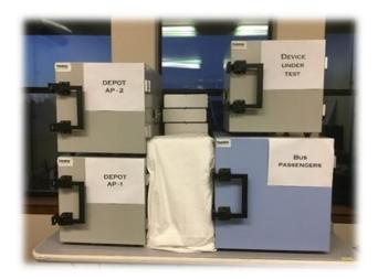
The example setup includes 4 RF chambers. Chamber 1 has a LANforge system that can emulate 100s of passengers in the bus, chamber 2 has the Device Under Test (the AP in the Bus) and chamber 3 and 4 have LANforge systems that emulate two APs in the depot. Third-party APs can also be used for the depot APs.
