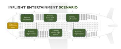
This example scenario uses 6 dual band LANforge systems to create 240 passenger stations in a simulated flight environment. All 240 stations are configured to download a video file over TCP representing the video streaming from a video server.
