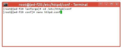
B. ...bind to a specific IP address, which is a good option if you configure the LANforge computer to have a fixed IP address on the management port. You would edit httpd.conf and change Listen to that specific IP address and port 80. Example: Listen 192.168.1.40:80
