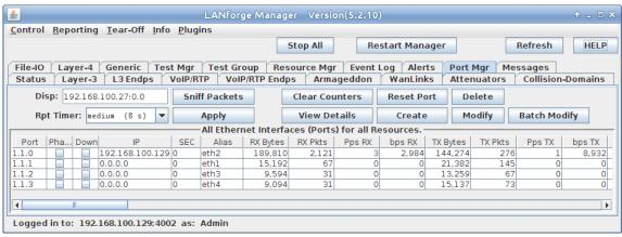
B. Modify port for Endpoint A (eth3). Set a valid network IP Address and Gateway IP.
