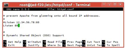
3. The demonstration test we'll create is making two ports, one for making requests and the other one for serving the protocol. Let's create two ports:
