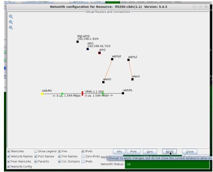
A. **NOTE:** The new connection is created and has a Bridged Mode WanLink between Redirect Device ports 1B and 2B which are shown as smaller, green squares (B-Ports) connected by a vertical bar (WanLink).
