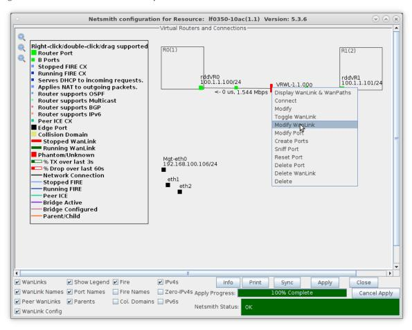
B. Verify that the B-side ports, rddVR0b and rddVR1b are filled in.
