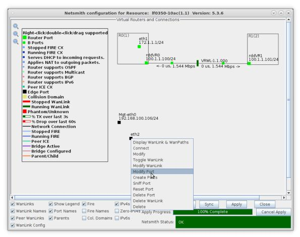
E. Assign port eth2 an IP address and Network Mask.
