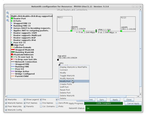
B. Assign port eth1 an IP address and Network Mask
