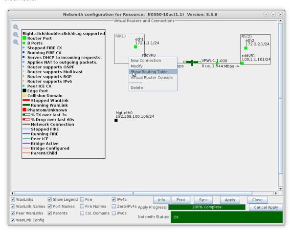
C. LANforge Virtual Routers by default use simple subnet routing, but can also use OSPF or BGP routing protocols. LANforge can also perform IPv4 multicast routing.
