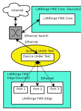
LANforge FIRE supports multiple Ethernet interfaces. To the System Under Test, it appears as if each interface is a separate PC or network appliance generating independent stateful traffic streams.
