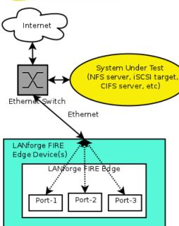
LANforge FIRE supports multiple Ethernet interfaces. To the System Under Test, it appears as if each virtual and physical interface is a separate PC or network appliance generating independent stateful traffic streams.
