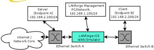
This diagram shows how one might use LANforge ICE to emulate a Wide Area Network between a Server and Client. When the Client communicates with the Server, the traffic will flow through the Ethernet switches and then through LANforge ICE. LANforge ICE will enforce the rate limitation and other network emulation as configured. The Client and Server are on the same subnet. For a simpler configuration, the Client and Server can be directly connected to the LANforge ICE system.
