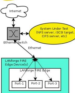
LANforge FIRE supports multiple Ethernet interfaces. To the System Under Test, it appears as if each virtual and physical interface is a separate PC or network appliance generating independent stateful traffic streams.
