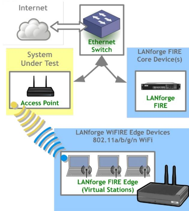
LANforge WiFIRE supports 802.11 Virtual Stations and Access Points\*. To the System Under Test, it appears as if there are multiple PCs sitting inside the LANforge system generating independent traffic streams over Wireless NICs.
