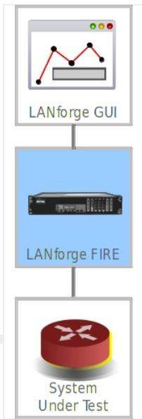
1. Connect one LANforge-FIRE port to the router's LAN port.
