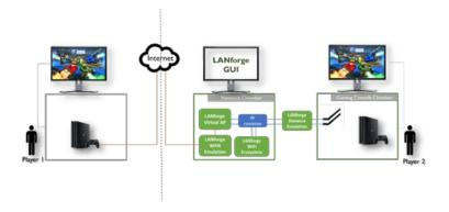
More advanced systems can support many concurrent and individually configurable network emulations by using many vAP interfaces paired with WAN emulation in the LANforge system.
